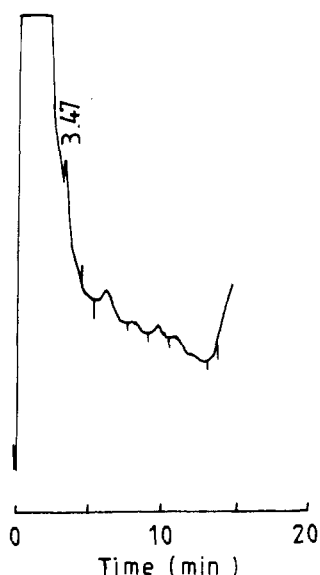
Figure 7. Chromatogram of control pork fat sample [injection of 2.5 \mu L of eluate 2 (4.8 mL) from 20 g of fat; column wide-bore HP 1, 240 ^{\circ} C].
